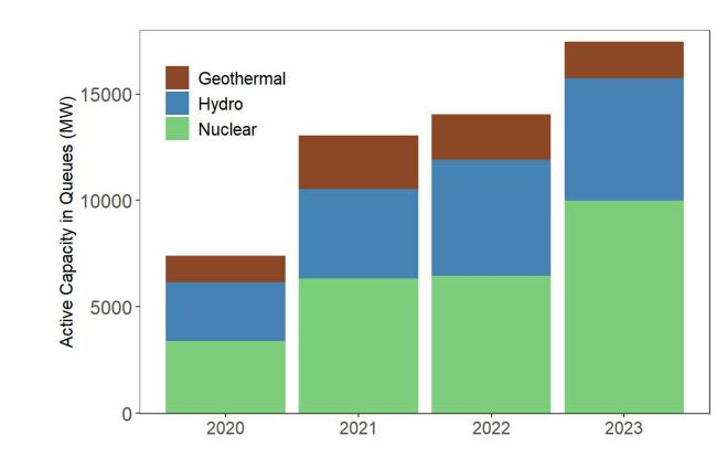
Active Nuclear capacity seeking grid connection increased to 10 GW in 2023 (up from ~6.5 GW in 2022), while Hydropower capacity held steady at ~5.7 GW. Geothermal capacity contracted slightly to 1.7 GW (from 2.1 in 2022).
