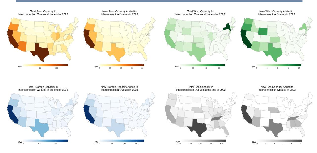
The mean Solar plant requesting grid connection in 2023 was 193 MW, >250% larger than in 2015; proposed Wind (+66%) and Battery (+330%) plants have also grown since 2015
