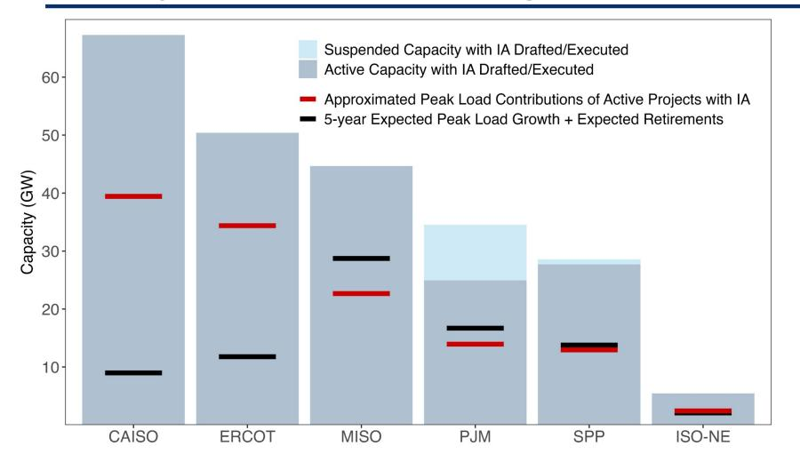
While total capacity of generators and storage active in interconnection queues provides an indication of longer-term developer interest in grid expansion, it provides less insight into shorter-term resource adequacy concerns related to power plant retirements and/or load growth that is being driven by transport electrification, manufacturing growth, and centers. Signed interconnection data agreements provide a better understanding of the nearer-term pipeline of project development (see graph).
