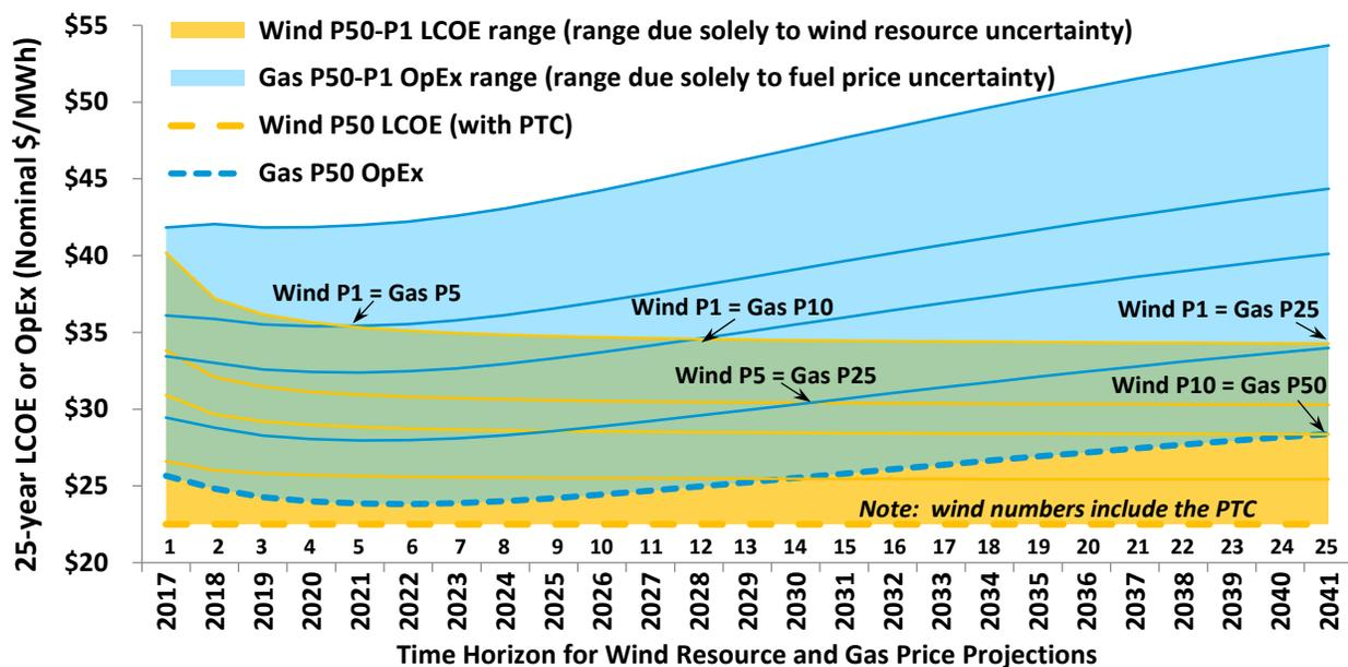
**Figure 10. P50-P1 wind LCOE (with PTC) and gas-fired OpEx over different time horizons**
