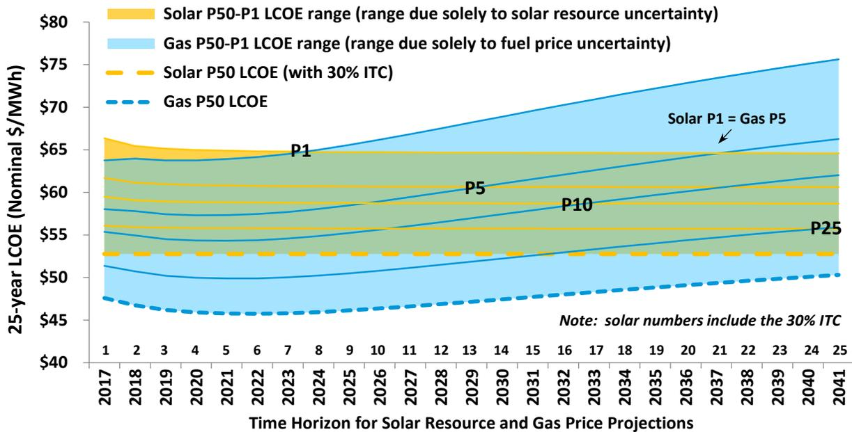
**Figure 11. P50-P1 solar (with 30% ITC) and gas-fired LCOE ranges over different time horizons**
